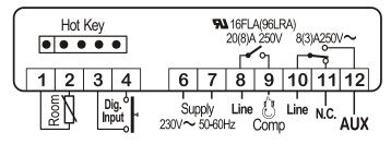
NOTE: In model with 110Vac the power supply has to be connected to 6-7 terminal NOTE: The compressor relay is 20(8)A or 8(3)A depending on the model.
